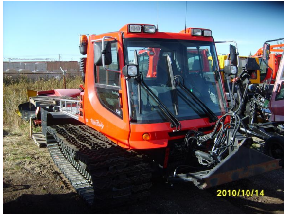
Pisten Bully PB100 Nordic Approx. 900 Hours 12-way blade Combi tracks Tiller with tracksetters
