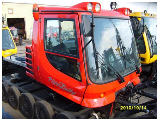
Pisten Bully PB200 Approx. 4600 hours 12-way blade 4.2 meter Combi tracks Fully reconditioned and painted
